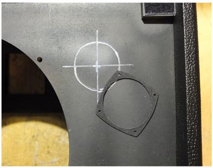
Drill the first hole with a wood drill. Align the drill so that the outer diameter of the drill tangents the circle from the inside. I used a 10mm wood drill here to demonstrate the process.
