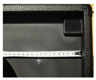
Drill the hole with the hole saw into the speaker baffle. Do not use to much pressure on the saw and lift the saw every so often to remove dust and splinters from the cutting area.
