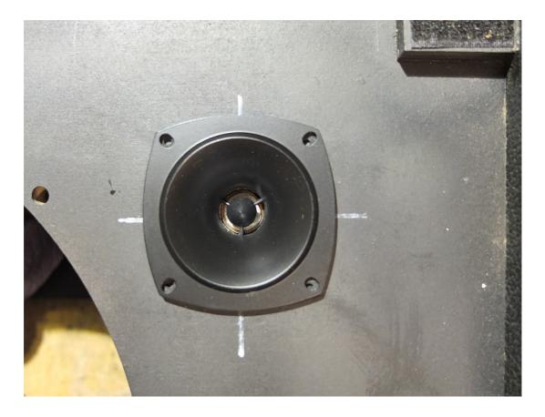
Please do not forget to put the rubber foam seal ring between the tweeter and the baffle.
