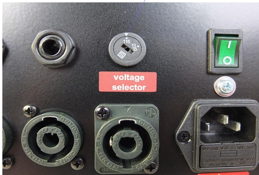
2. **Disconnect the power cord from the Amplifiers mains input socket !**
