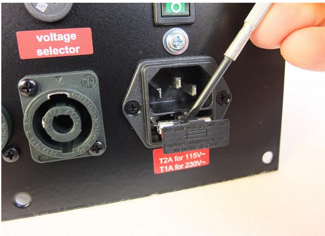
The fuse closer to the socket is the active fuse. The fuse at the outside of the fuse holder is a spare fuse.
