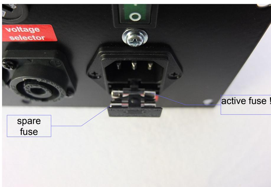
**The Camplifier will come with the correct fuse inserted in the active position according to the mains input voltage selection your Camplifier comes with.**
